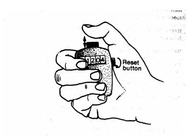
Figure 3: Tally counter used for accurately counting waterbird flocks.
