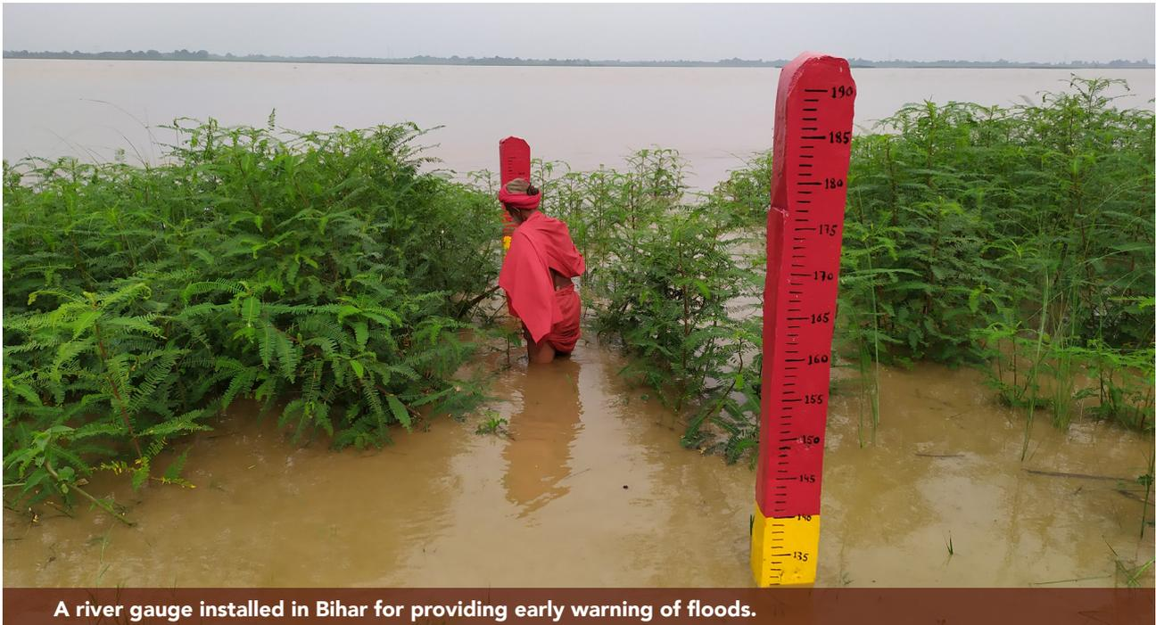
A river gauge installed in Bihar for providing early warning of floods.
