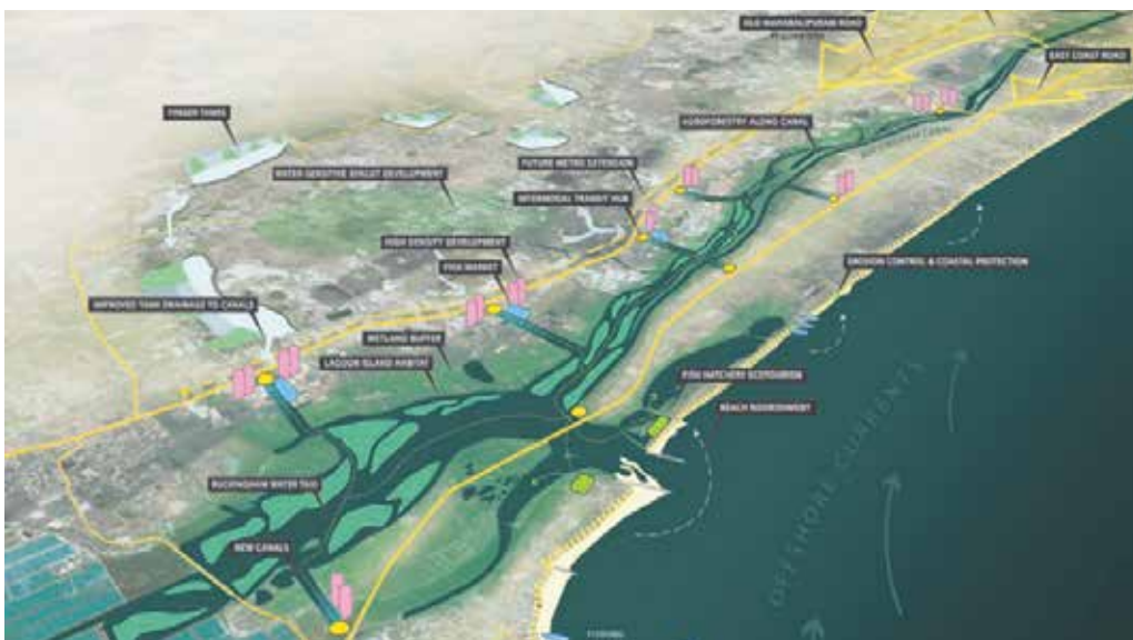
A model design for Muthukadu basin straddling the southern boundary of Chennai. The model, developed by Deltares team shows how wetlands can be used as coastal defense
